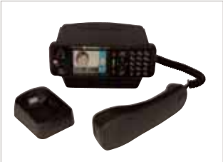
GMMN1006 Telephone style handset for transmit or receive communications with push-to-talk and volume control. For use with junction box GMLN3002.
