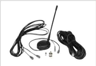
GMAE4293 Combined TETRA and GPS antenna for digital car kit with 440-470MHz frequency range including duplexer and DC adapter. Compatible with car kit FTN6307.
